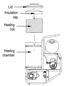
Figure 20 – Heating Chamber Interior
