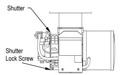
Figure 25 – Shutter Adjustment
